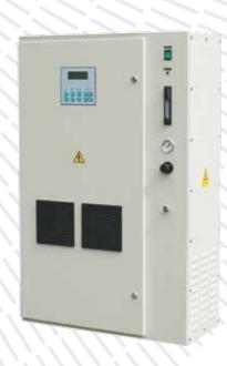
The ozonia® TOGC8X, 13X & 45X ozone generators are wall-mountable, aircooled units specifically designed for industrial use. The system incorporates function indicators, feed gas flowmeter, oxygen concentrator and variable output control.
