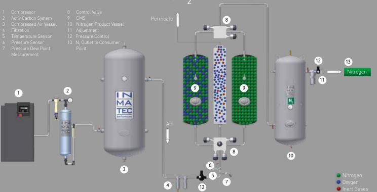
The Pressure-Swing-Adsorption (PSA)-technology is based on the adsorption principle, using a carbon molecular sieve (CMS) as adsorbent.
